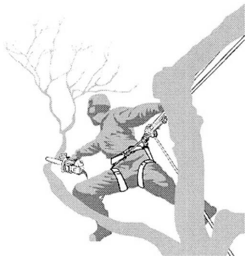
SB5 - Example of one-handed chain-saw use
