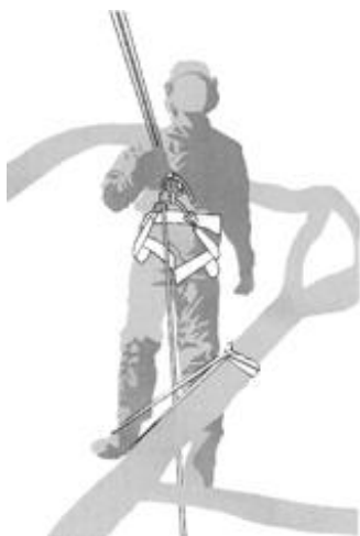
SB4 - Example of temporary foot stirrup created from endless sling
