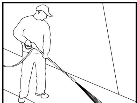
Figure 6 – Optimal angle to cleaning surface
