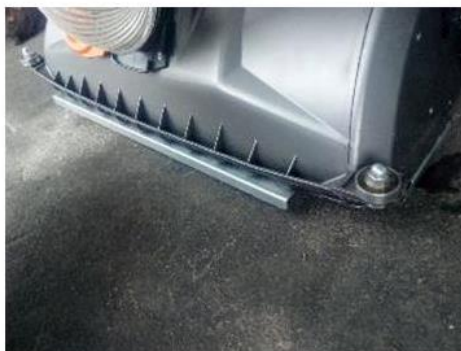
Fig. 30-2 The baffle is inserted into place
