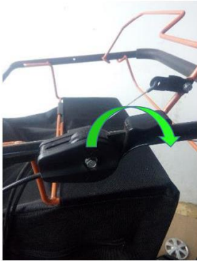
Fig. 38 Handle off position
