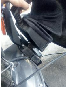
Fig. 37-1 Take down the bag interface
