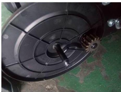
Fig. 39-1 Add grease to the gear
